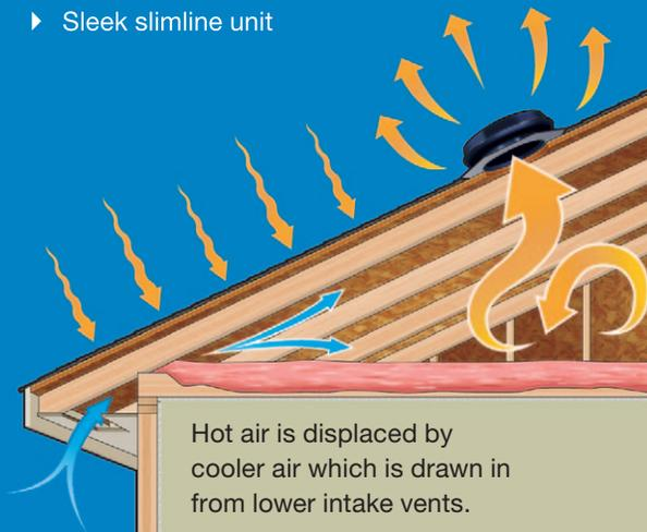
Hot air is displaced by cooler air which is drawn in from lower intake vents.
