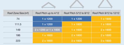
Recommended air intake venting (eaves or soffits) size requirements:
