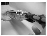
Pull the side controller off the motor strip.
