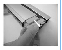
Fit the new side controller on the motor strip.
