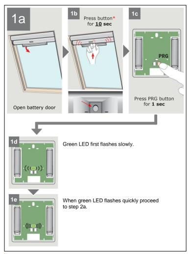
\* blind button is found inside the battery cavity – behind the aluminium fascia.
