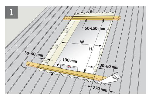
Cut the metal sheets taking care to maintain the correct distance from the course of metal sheets to skylight frame. Overcut at both sides below skylight to allow for full width of apron to come through metal sheet.
