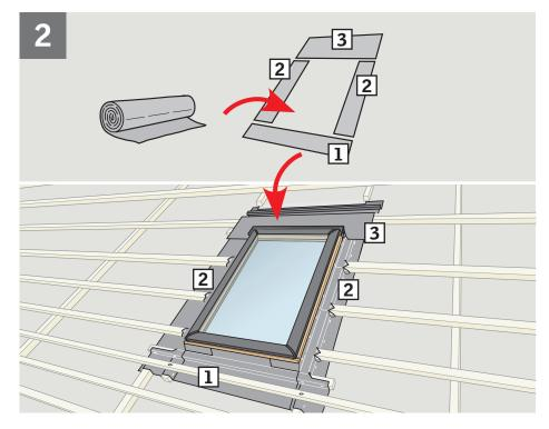
If roofing underlay is used (provided by installer): Dress roofing underlay up around all four sides of the frame. Roof with counter battens shown for illustration purpose.
