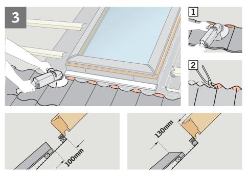
1 Tiles or 2 metal roof should be chamfered if necessary.
