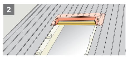
This top flashing section under the existing metal roof before laying the skylight in position. Take care to maintain 30-60 mm distance from sides of frame to metal roof, 100 mm below and 60-150 mm above skylight.
