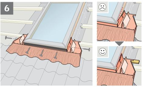
Position bottom flashing section as shown and install battens to support joints with side flashing sections if necessary.
