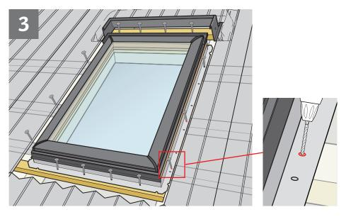
Check level at bottom of frame and fix the angle brackets on the skylight to the rafters .
