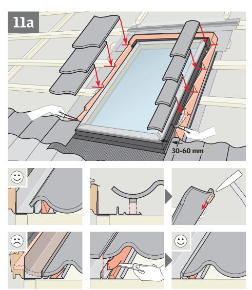
Trim foam gasket and flatten upstands on side sections as necessary. Make a slit above each tile to allow foam gasket to seal against underside of tile. Maintain distance to frame as shown; cut tiles if necessary. To make tile lie correctly it may be necessary to remove neck on tile and flatten the returned edge around the battens.
