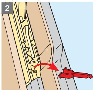
**ENGLISH: Connection of springs with fittings:** Push sash upwards, ensuring that fittings and springs on both sides automatically connect **1**. Then pull sash downwards slightly to remove red plastic clips **2**.
