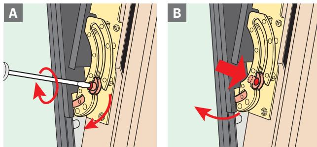
**ENGLISH: Remove window sash.** Hinges may either have a screw A or a push button B. Press in push button, eg with a screwdriver.
