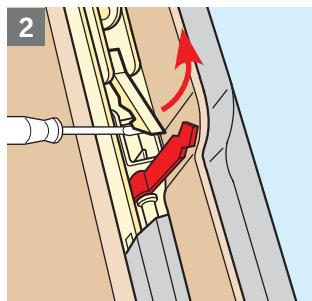
**ENGLISH: Disengage springs:** Open window, pull sash downwards a little and insert red plastic clips **1**. Push sash upwards and disengage hooks **2**.
