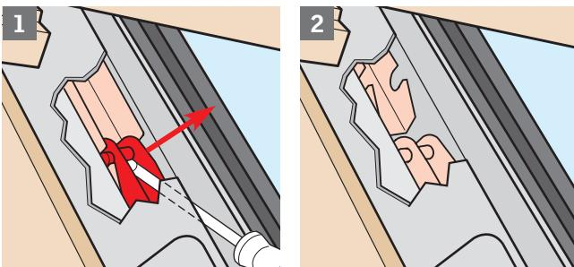
**ENGLISH: Disengage springs:** Open window. Push sash upwards and tip up sliding devices 1, 2.
