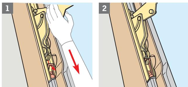
**ENGLISH:** Push sash upwards, while pulling fittings downwards to connect with springs on both sides **1**, **2**.
