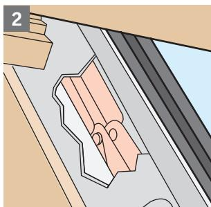
**ENGLISH: Connection of springs with fittings:** Push sash upwards, ensuring that fittings and springs on both sides automatically connect **1**, **2**.
