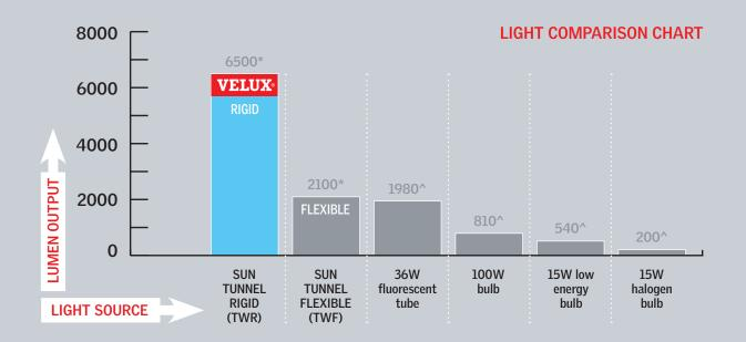
Please note: Light transmittance of VELUX Sun Tunnels depends on parameters such as sky conditions (cloudy/sunny), direction of sun light, orientation and length of Sun Tunnel. VELUX Sun Tunnels in this chart have been tested with a 1 metre shaft, on a 15° roof pitch in summer, at noon on a sunny day using a photometer. (TWR rigid tunnel emits 440 lumens when measured on a cloudy winter's day).
